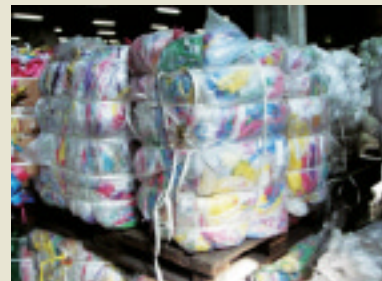
Compressed waste plastic blocks Waste plastics are compressed so that IC tags can be attached.
